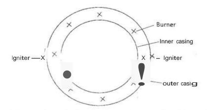
This type of combustion chamber consists of a single flame tube completely annular in form, which is contained in an inner and outer casing. The burners are suspended in the annular for supplying the fuel from the fuel manifold. There are two igniter plugs, one on each side of the engine.
