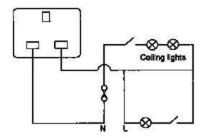
(i) Point out two faults in the circuit.
