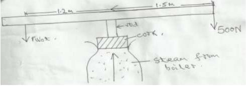
If the area of the cork is 15cm<sup>3</sup> and a force of 500N is needed to keep the cork in place, determine the pressure of the steam in the boiler. (3 marks)
