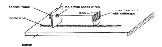
b) Adjust the position of the lens arrangement (lens, mirror and holder) until a sharp image of the cross-wires is observed on the screen O.
