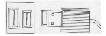
USB port and its interface USB is set to replace the convectional parallel and serial cables and port It provides very high speed and quality data transmission over distance by approximately 5 meters
