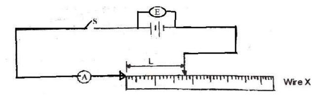
b) Measure the voltage, E before closing the switch
