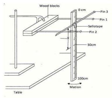
c) Displace the lower end of the metre rule slightly and let it oscillate as shown in the figure above. Measure and record in table below the time t(s) for 10 oscillation (d) Repeat procedure in (b) and (c) above for the values of X shown in the table and fill and complete the table.
