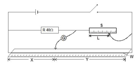
c) Close the switch and use the jockey to touch one end of the wire W, and then the other end. The deflections on the galvanometer should be in opposite directions, if not check the circuit. Adjust the positions of the jockey along the wire W until there is no deflection in the galvanometer. Record the value of x and y.
