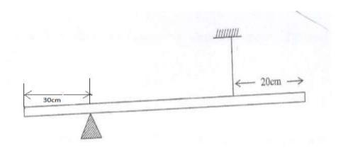
Given that the weight of the bar is 1.5N, determine the tension in the string. (3 marks)
