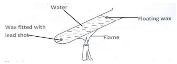
The boiling tube was heated in the middle as shown.
