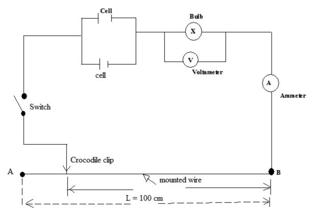
b) With the crocodile clip at A (ie L = 100cm) take the voltameter reading (V) and the ammeter reading (I). Record V and I in the table below.
