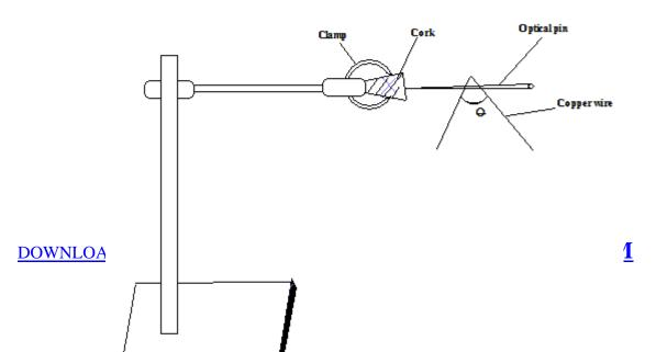
c) Give it a small displacement so that it oscillates about a point on the pin. Measure the time, t(s) for 10 oscillations of the wire.
