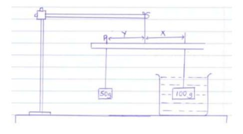
c) Calculate the apparent weight of the 100 g mass in water. 3mk)
