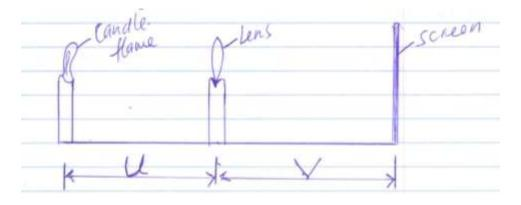
b) Set the position of the lens so that the 40cm from the candle (U=40). Adjust the position of the screen until a sharp image of the candle flame is obtained. Measure the distance, V between the lens and the screen. Record the value of  $V_1$   $V = \dots cm$  1mk)
