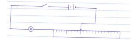
b) Measure the voltage, E ( across the cells) before closing the switch -
