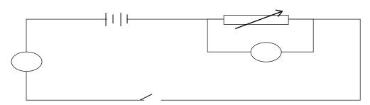
b) Adjust the potentiometer until you are able to obtain minimum reading on the voltmeter and maximum on the ammeter. Record these readings in the table below.
