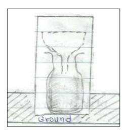
The raingauge is dug into the ground as shown above.
