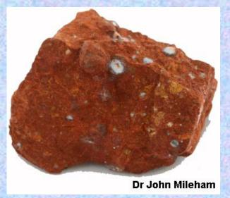
Aluminium ore (bauxite) has a very high melting point (2050°C).
