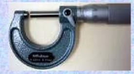
A micrometer screw gauge is used to measure small lengths ranging between 0.10 mm and 25.00 mm.
