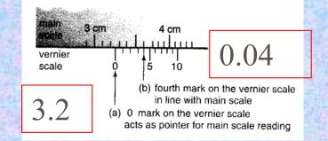
(c) The reading of the vernier caliper is the result of the addition of the reading on the main scale to the reading on the vernier scale.
