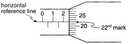
11 Readings on the micrometer are taken as follows.
