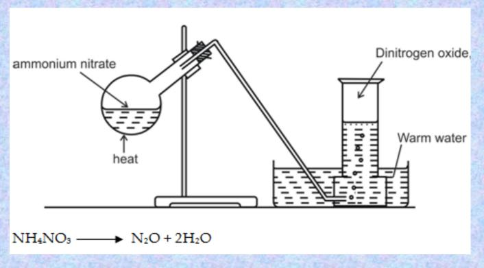
Nitrous oxide is a linear molecule. It has a boiling point of -88 °C, and a melting point of -102 °C. It is colourless and has a faintly sweet smell. It is used as an anesthetic, popularly called laughing gas.
