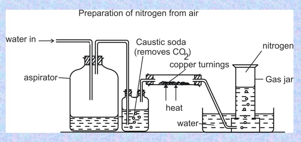
Nitrogen can be prepared from the air as shown. Air flows into the respirator and onto caustic soda which dissolves carbon dioxide gas.
