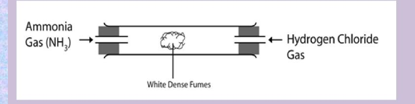
Ammonia diffuses faster and white dense fumes will be formed near hydrogen chloride gas – the white dense fume is ammonia chloride.
