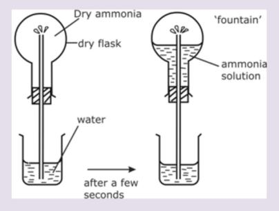
As soon as this water enters the flask, the ammonia dissolves in it, forming a partial vacuum. As a result of it, water rushes in and comes out of the tube as a jet of fountain.
