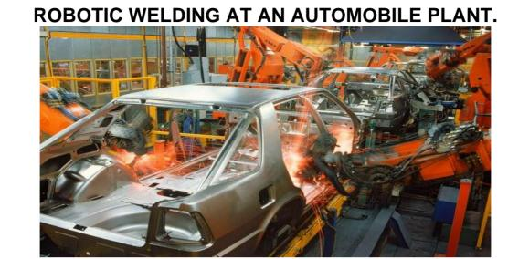
In the final assembly line one can see clearly how machinery and human effort in assembly are divided into many specialized skills. The special tooling and machinery developed to handle assembly parts and to aid operators in their tasks can also be observed.
