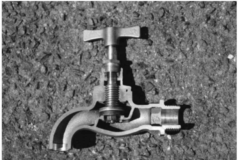
Figure 5.3.2: A cross section through a tap
