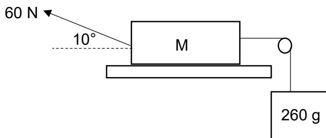
A force of 60 N is applied to the stationary block on the table at an angle of  $10^\circ$  to the horizontal. It causes this block to accelerate at  $2.89 \text{ m}\cdot\text{s}^{-2}$  to the left. The coefficient of kinetic friction between the block and the surface of the table is 0.3. Ignore the effects of air friction.
