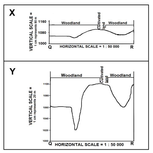
2.3.1 Match cross-sections **X** and **Y** with the vertical exaggerations below.
