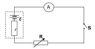
The learners use their recorded readings of current and resistance, together with the equation  $R = \frac{\epsilon}{T} - r$ , to obtain the graph below.
