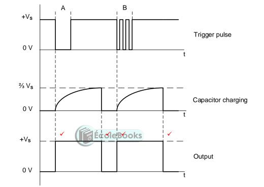
NOTE. Inverted polarity with correct intervals minus two marks
