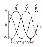
**NOTE:** The sequence of R,Y,B  $(V_{L1}, V_{L2}, V_{L3})$  must be correct to be awarded full marks
