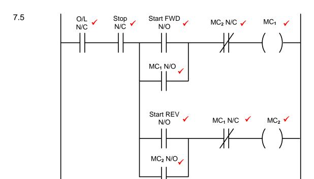
**NOTE:** O/L and Stop must both be in the same condition (either open or closed)
