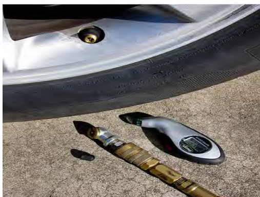
Two more complicated types of tyre pressure gauges for measuring the air pressure inside car tyres. The right one is a digital gauge.
