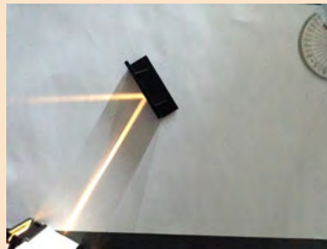
A mirror is placed on the line and a ray shone to strike the mirror at the normal line.
