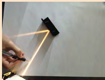
Marking the incident light ray.
