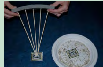
Now you can see how a telescope's mirror can collect lots of light and direct it into a small detector, like your eye.
