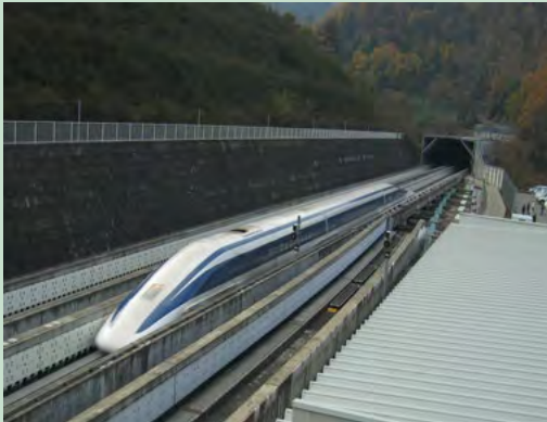
Japan's high speed train the JR-Maglev MLX01 has reached 581 km/h.
