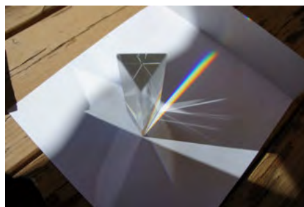
Refraction through a triangular prism.
