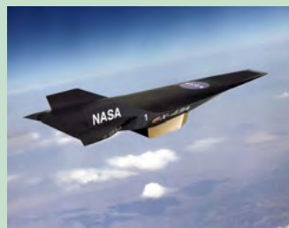
NASA's scramjet the X-43 flies at 7000 km/h.
