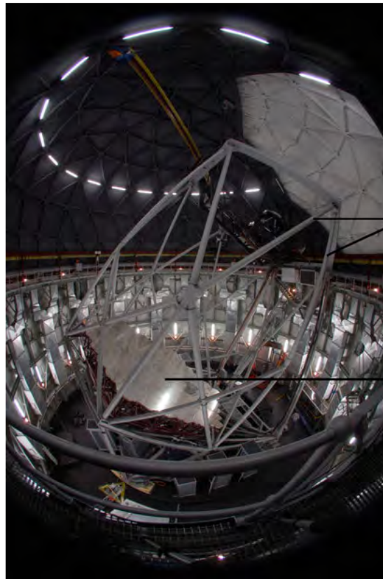
SALT's giant mirror, made up of 91 individual mirrors.
