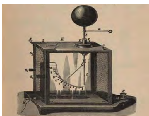
An early example of an electrostatic induction demonstrator with one gold strip at the bottom and a ball at the top.
