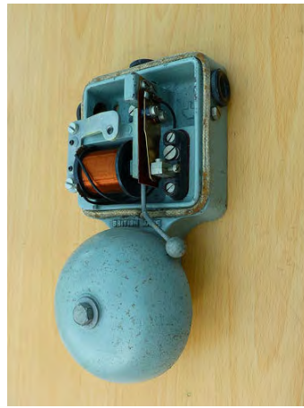
An electromagnet in a bell.
