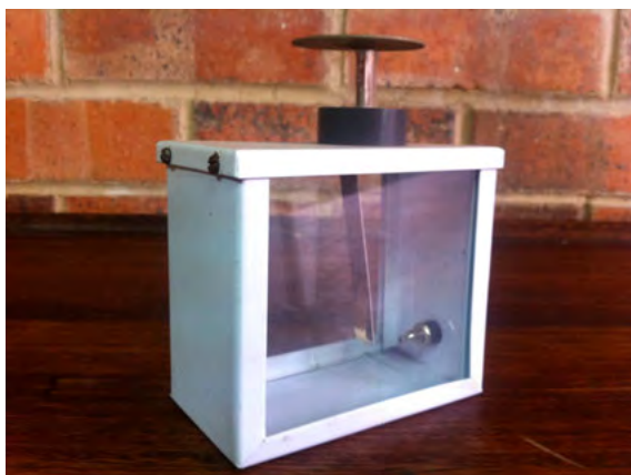
An electrostatic induction demonstrator used in a laboratory.
