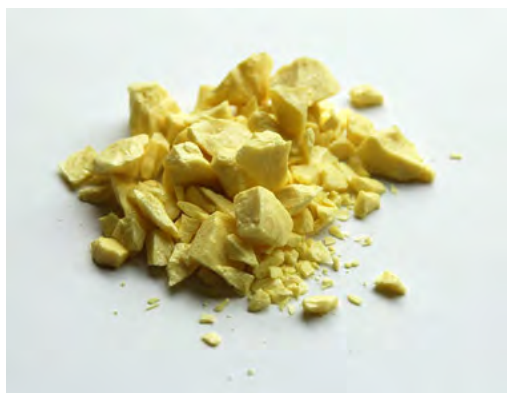
Sulfur is a yellow substance and it burns with a blue flame in oxygen.
