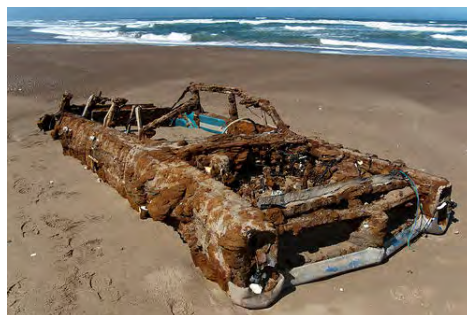
An abandoned car quickly rusts and corrodes near the sea.
