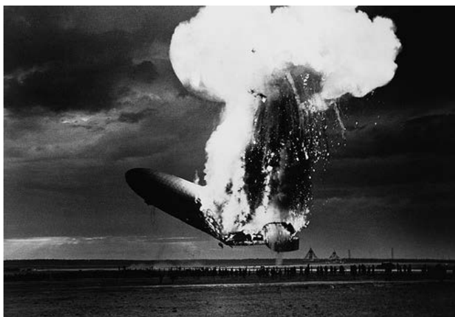
In 1937, a German airship exploded and fell to the ground in a huge fireball as the hydrogen gas which kept it floating ignited and reacted with the oxygen in the air.
