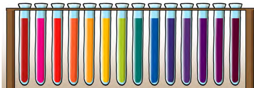
Universal indicator can have many different colours, from red for strong acids to dark purple for strong bases. The liquid inside the middle test tube is neutral (pH = 7) and this is shown by the green colour of the indicator.
