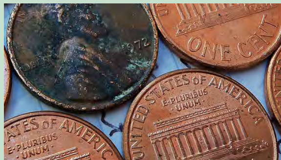
One of these copper coins is tarnished as it has become coated in a black substance.
