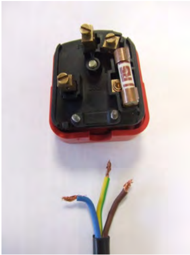
The three wires that form the cable leading to a plug.
