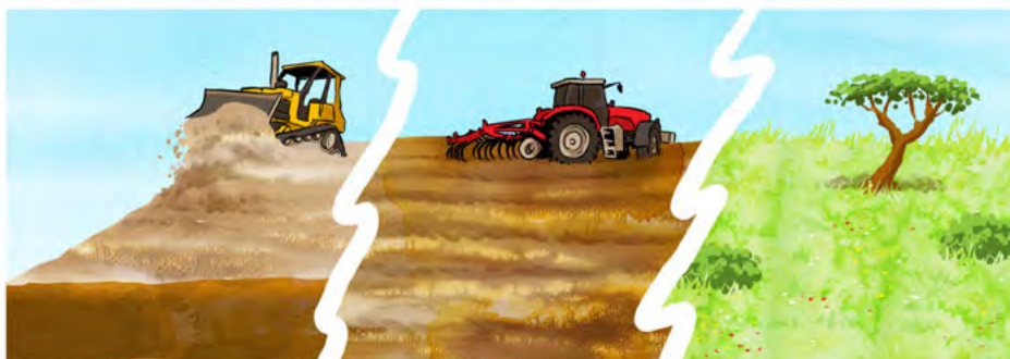
Replacing the overburden and topsoil
