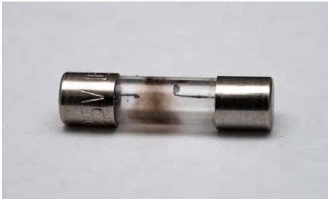
This fuse has blown and has to be replaced.
