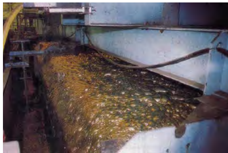
Separating minerals by flotation
