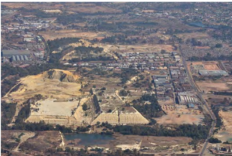
An aerial photograph of Primrose Gold Mine. Can you see the piles of gold tailings on the left of the photograph?
