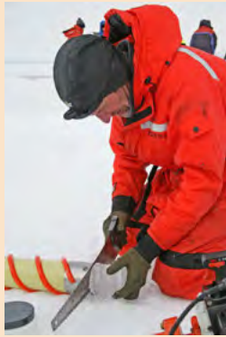
Sawing through the ice core to obtain samples for analysis.
