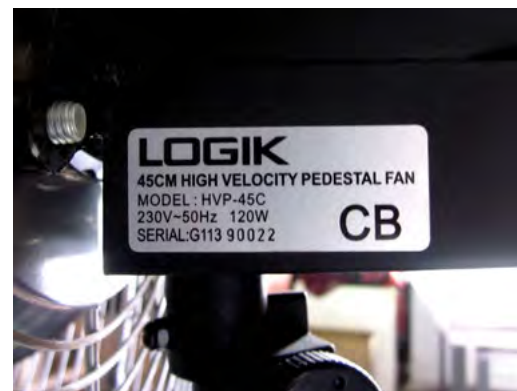
The label on a fan indicating a power rating of 120 W.
