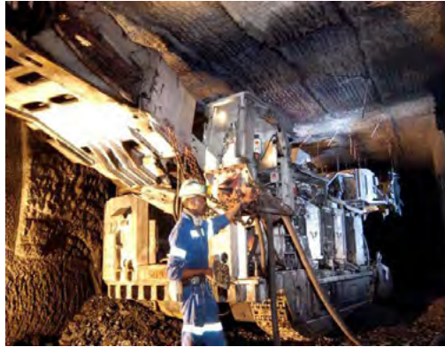
A machine called a continuous miner at work at the coal face.
