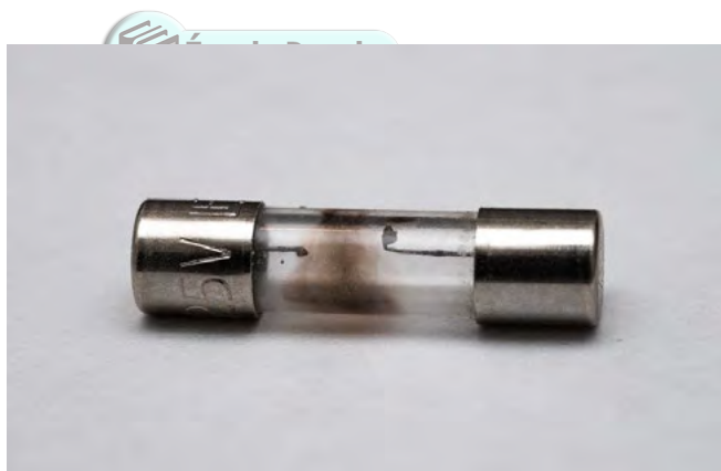
This fuse has blown and has to be replaced.
