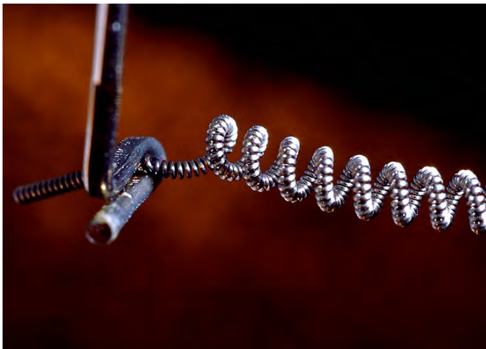
A close-up photograph of the tungsten filament in an incandescent light bulb.
