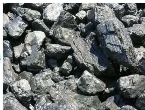
Lumps of coal can be used directly as a fuel. However some coal is first washed to make it into 'high grade coal'. It can also be sorted into various sizes, depending on what the fuel is required for.
