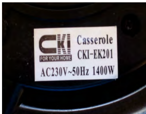
The label on an electric pan indicating a power rating of 1400 W.
