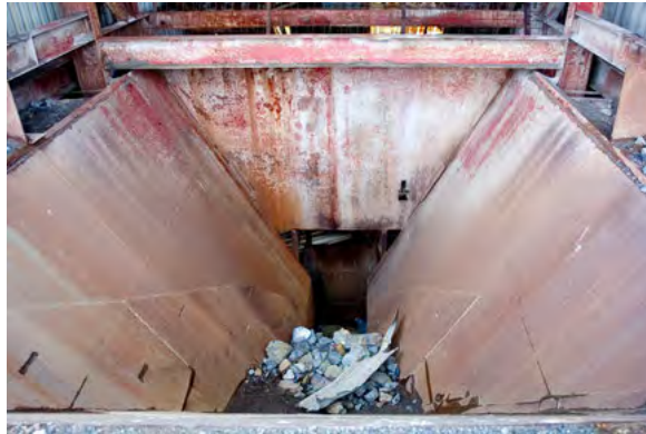
Jaw crusher at a mine. The rocks are fed into the funnel and crushed as the two sides move back and forth.
