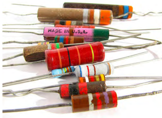
Different types of resistors used to add resistance to an electric circuit.
