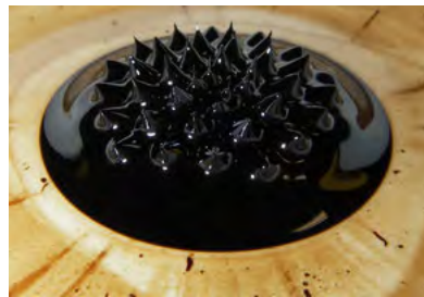
An example of a ferrofluid, a liquid that can become magnetised in a magnetic field.
