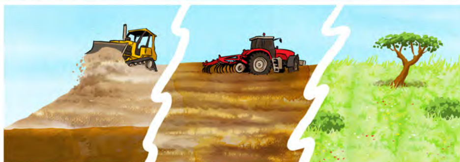
Replacing the overburden and topsoil
