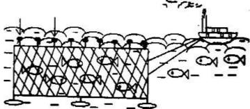
Purse seining net method: this involve the use of two boats called seine boats. The net is laid out in a circle to surround a shoal of fish attracted by an echo sounder. At the bottom of the net there are rings attached
