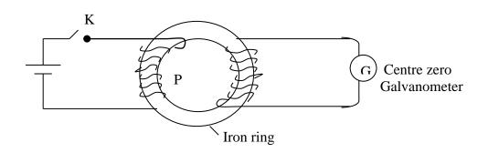
The diagram in the figure above shows a model of a transformer in which the primary coil P is connected to a d.c. source and the secondary coil S is connected to a galvanometer.
