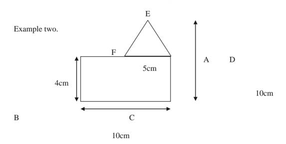
The figure shows a uniform composite lamina made of a rectangle ABCD and an isosceles triangle DEF. Find the position of the centre of gravity.
