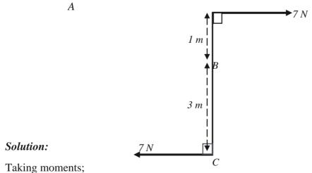
About A: Moments =  $(7 \times 4) + (7 \times 0) = 28$  Nm *Clockwise* About B: Moments =  $(7 \times 3) + (7 \times 1) = 28$  Nm *Clockwise* About C: Moments =  $(7 \times 4) + (7 \times 0) = 28$  Nm *Clockwise Observation:*  Three or more parallel forces may also form a couple.
