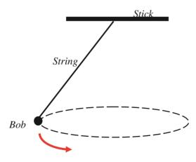
As the bob describes a horizontal circle, the string also describes a curved surface of a cone hence this system is referred to as a **conical pendulum**.
