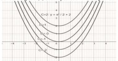
The general solution represents all the curves with similar variable term but different constants as shown in the diagram.
