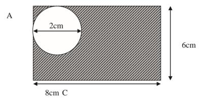
The shaded area shows a uniform rectangular laminar with a circular hole. Find the centre of gravity of the laminar.
