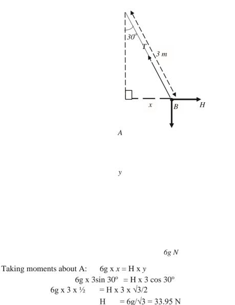
To find the Tension in the string, we apply Lami's theorem of three forces in equilibrium:
