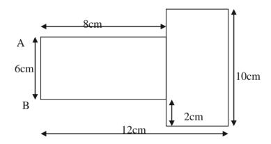
The figure shows a uniform composite lamina. Find the position of the centre of gravity. Let the mass per unit area be  $\rho$ .
