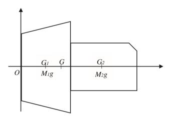
Lamina 1 has mass  $M_1$  and C.O.G  $G_1$ Lamina 2 has mass  $M_2$  and C.O.G  $G_2$ Composite laminae has mass  $(M_1 + M_2)$  and C.O.G as G.
