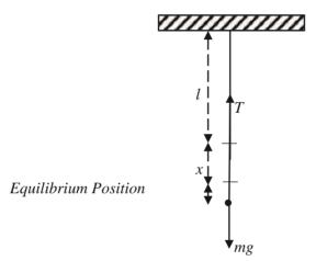
The string gained potential energy due to gravity when we attached the stone hence the first extension *x*. When we pull down the stone then release it, it moves back to its *equilibrium position* where it was hanging freely. The kinetic energy at a certain velocity causes the movement back to the equilibrium position.
