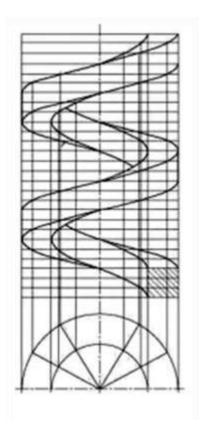
The insertion of a core makes it a thread as indicated below. Draw two turns of the thread below using the given specifications.
