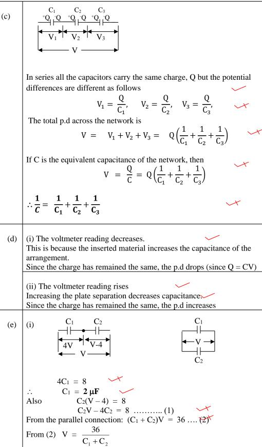
Substituting for V in (1), we have  $\frac{36C_2}{C_1 + C_2} - 4C_2 = 8$
