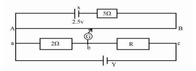
In the figure above AB is a uniform wire of length 100cm and resistance  $10\Omega$ . X is a driver cell of e.m.f 2.5V and negligible internal resistance. When the galvanometer G, is connected in turn to points b and c, the balance lengths are, 64.0cm and 90.0cm respectively. Calculate the;
