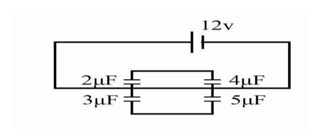
The figure above shows a net work of capacitors connected across a battery of e.m.f 12*V*. Calculate the:
