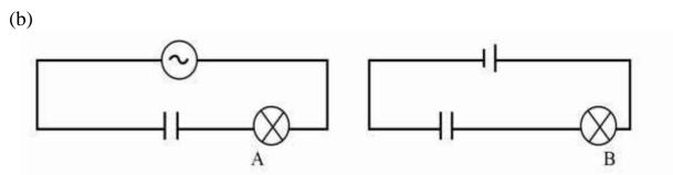
In the figure above, the bulbs A and B have the same ratings. A is connected in series with a capacitor across an a.c source while B is connected in series with
