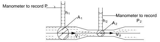
Consider the fluid to be non viscous, incompressible and of density  $\rho$  in a horizontal steady flow let the pressure and velocity be  $P_1$  and  $V_1$  at the main pipe and  $P_2$  and  $V_2$  at the constricted pipe along the same stream line
