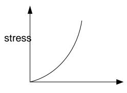
Rubber stretches very easily without breaking and has a greater range of elasticity. Rubber is much less stiff than metals and therefore its value of young's modulus is very much smaller than that of most metals. It does not undergo plastic deformation. Un stretched rubber has coiled molecules and when stretched they
