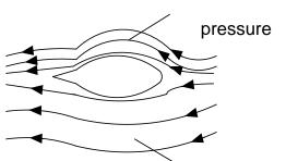
so that air flows faster along the top of the wings than below the wings.
