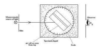
The air cell is immersed in a liquid under test. A beam of monochromatic light is
