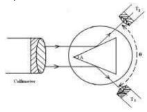
With the table fixed, the telescope is moved to position  $T_1$  to receive the light from the collimator on its cross wire. This position  $T_1$  is noted and the telescope is turned n to a new position  $T_2$  to receive light on its cross wire. The angle  $\Box$  between  $T_1$  and  $T_2$
