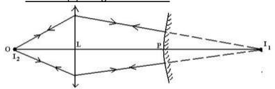
An object 0 is placed in front of a convex lens to form a real image on the screen at I<sub>1</sub>.
