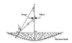
A small quantity of the liquid under test is poured into a concave mirror of known radius of curvature r. An object pin is moved along the principal axis of the mirror until it coincides with its image at I. The distance IP is noted. The required refractive index  $n_1 = \underline{r}$
