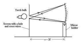
An illuminated bulb, a screen and a concave mirror mounted in a holder are aligned as shown above. The mirror position is adjusted to or from the screen until a sharp image of the cross-wire is formed on the screen besides the object.
