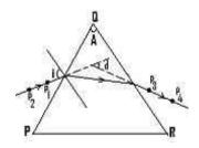
Two optical pins  $P_1$  and  $P_2$  are placed along the lines that make different angles of incidence i. Pins  $P_3$  and  $P_4$  are placed such that they appear to be in line with the images of  $P_1$  and  $P_2$  as seen through the prism. The angles of deviation d are measured for different angles of incidence. A graph of d against i is plotted to give a curve whose angle of deviation at its turning point is the angle of minimum deviation  $D_{min}$  of the prism.
