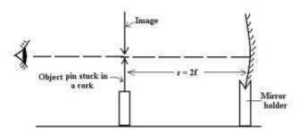
An object pin is placed in front of a mounted concave mirror so that its tip lies along the axis of the mirror.
