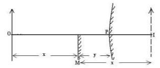
An object pin O is placed in front of a convex mirror and a virtual diminished image is formed at I. A plane mirror M is placed between O and P so as to intercept half the field of view of the convex
