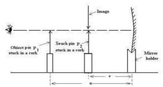
An object pin  $P_1$  is placed at a distance u in front of a mounted concave mirror so that its tip lies along the axis of the mirror.
