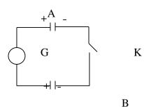
A ballistic galvanometer G, with sensitivity of 2 divisions per  $\Box C$  joins the positive plates of the capacitors. If K is now closed, what will be the throw on G? (5) 4(a) (i) State Coulomb's law of electrostatics. (1)
