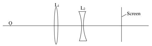
The arrangement casts a sharp image of O onto a screen which is 30 cm from L<sub>2</sub>. (i) Calculate the distance between the two lenses.
