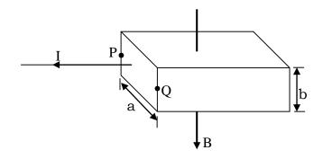
(i) Account for the occurrence of a potential difference between points P and Q, indicating the polarity of this p.d.
