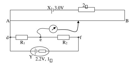
When the centre-zero galvanometer is connected in turns to points  $\mathbf{e}$  and  $\mathbf{f}$ , the balance lengths obtained are 45.0 cm and 80.0 cm respectively. Calculate the:
