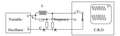
C is a capacitor and L an inductor. The output through C is connected to the  $Y_1$  plates while that through L is connected to the  $Y_2$  plates of a double-beam C.R.O.  $y_1$  and  $y_2$  are the respective signals due to the inputs at  $Y_1$  and  $Y_2$ . It is observed that as the frequency of the oscillator is varied from minimum to maximum the amplitude of  $y_2$ decreases as that of  $y_1$  increases. Explain these observations. (4)
