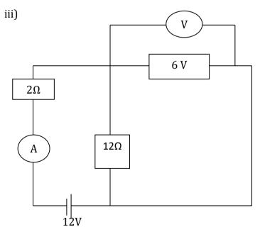
In the circuit above, the battery as negligible internal resistance. Find the ammeter and voltmeter readings. [4mks]
