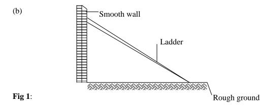
Fig 1 above shows a uniform ladder, 10m long and weight 100N leaning against a smooth vertical wall. The bottom of the ladder is 6m from the base of the wall. A man whose weight is 700N stands on the ladder at a point 6m above the ground. Calculate the forces acting on the ladder. (07 marks)
