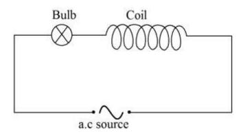
An air cored coil, a bulb and a.c source are connected as shown in fig 3 .When a solid iron core is introduced into the cool, the bulb becomes dimmer and the core hot. Explain the observation. (6mks)
