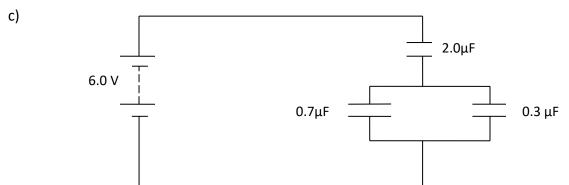
Three capacitors of capacitances  $0.7\mu\text{F}$ ,  $2.0\mu\text{F}$  and  $0.3\mu\text{F}$  are connected as shown in the figure above. Calculate the energy stored in the  $2.0\mu\text{F}$  capacitor when fully charged. (6mrks)
